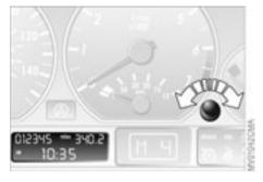
In ignition key position 0: the time is displayed for a few seconds after you press the left button, refer to Odometer on page 71.
